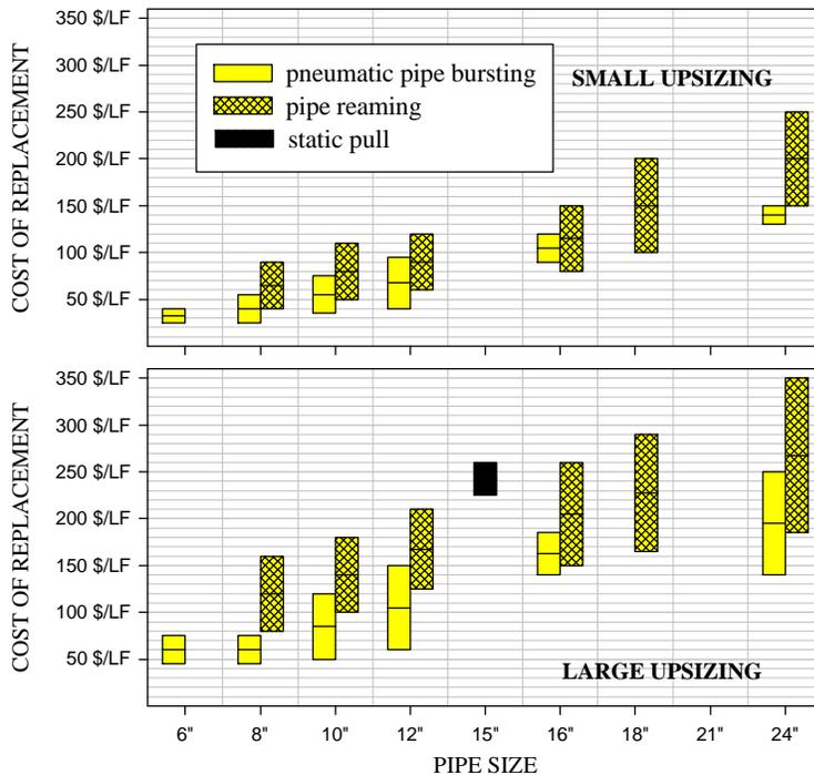
**Figure 1-15: Bid cost of pipe replacement with upsizing (1999).**
