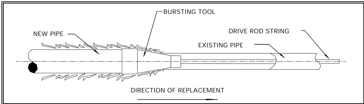
**Figure 1-5: Bursting head of the static pull system**
