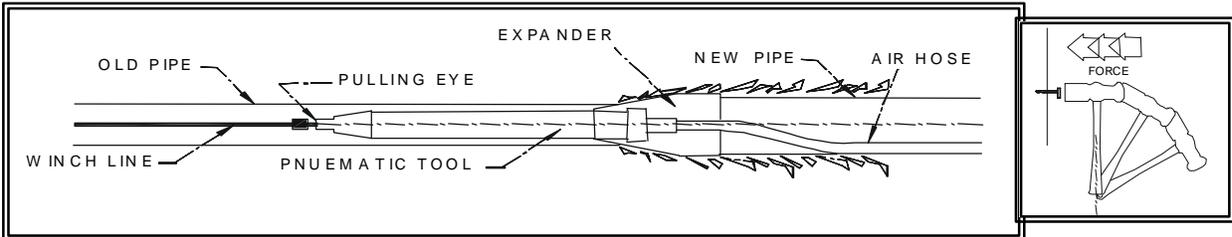
**Figure 1-3: Bursting head of the pneumatic system**
