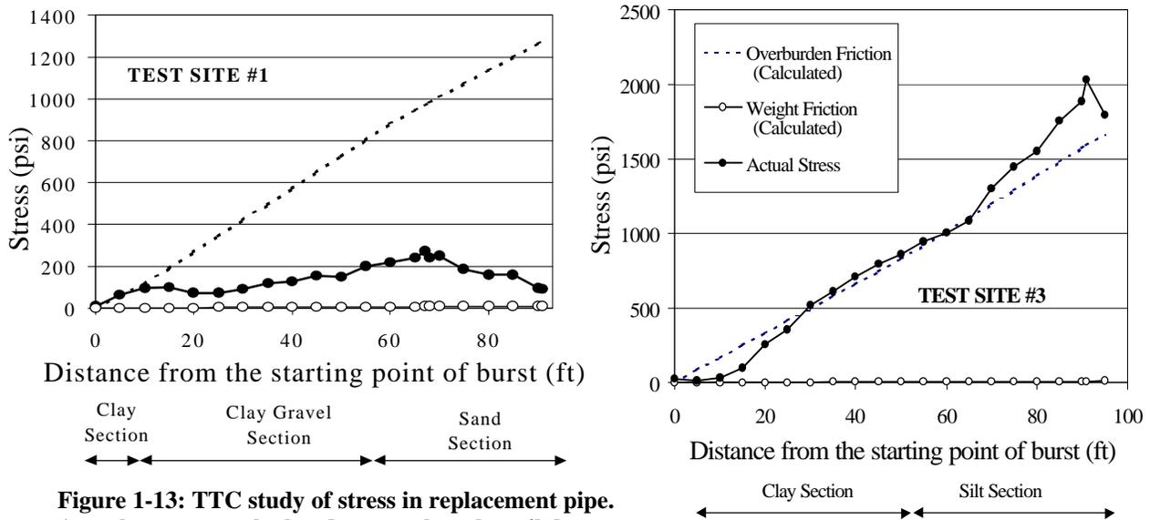
**Figure 1-13: TTC study of stress in replacement pipe. Actual stress vs. calculated stress when the soil does not collapse around the pipe (left) and when it does (right). (Atalah, 1998)**
