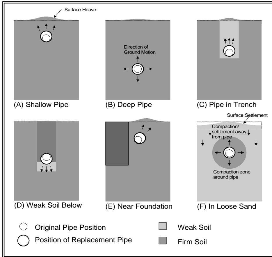
**Figure 1-11: Conceptual effect of site conditions on ground displacements**
