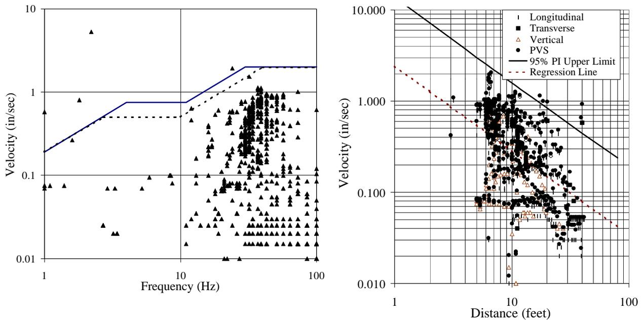
**Figure 1-12: TTC study of ground vibrations. Compiled peak particle velocity vs. frequency for all test sites (left). Velocity vs. distance from the bursting head for all test sites employing pneumatic system (right). (Atalah, 1998)**
