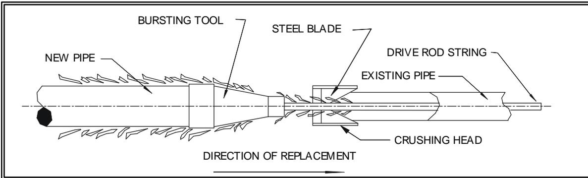
**Figure 1-6: The crushing head in implosion (IMPIPE System)**
