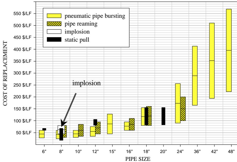
**Figure 1-14: Bid cost of size-for-size pipeline replacement (1999)**
